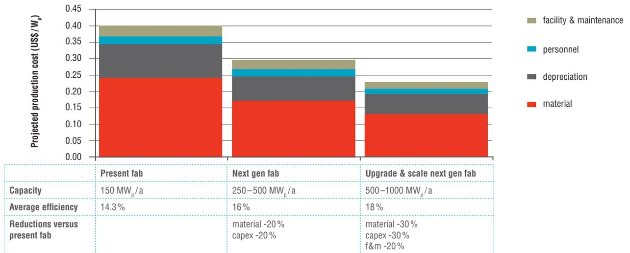
Fig. 3: Projected CIGS production cost using presently available technology and leveraging further cost reduction potential
