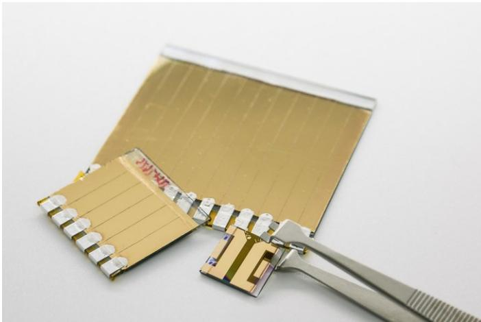
From the laboratory cell to a small solar module: A perovskite innovation from the ZSW laboratory. Photo: ZSW.
