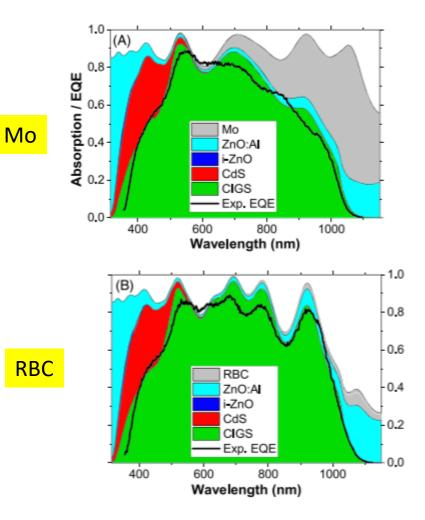
Voc = 644 mV Jsc = 28.9 mA/cm<sup>2</sup> FF = 72.7 % Eff = 13.5 % without ARC
